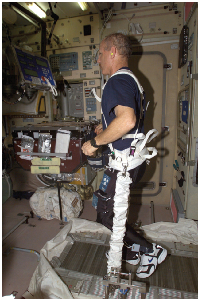
FIGURE 4.11 Astronaut Kenneth D. Bowersox, Expedition Six mission commander, wearing the Lower Extremity Monitoring Suit, participates in the Foot/Ground Reaction Forces During Spaceflight experiment. NASA Photo ID: ISS006-E-11016 (24 December 2002). SOURCE: Courtesy of NASA.
