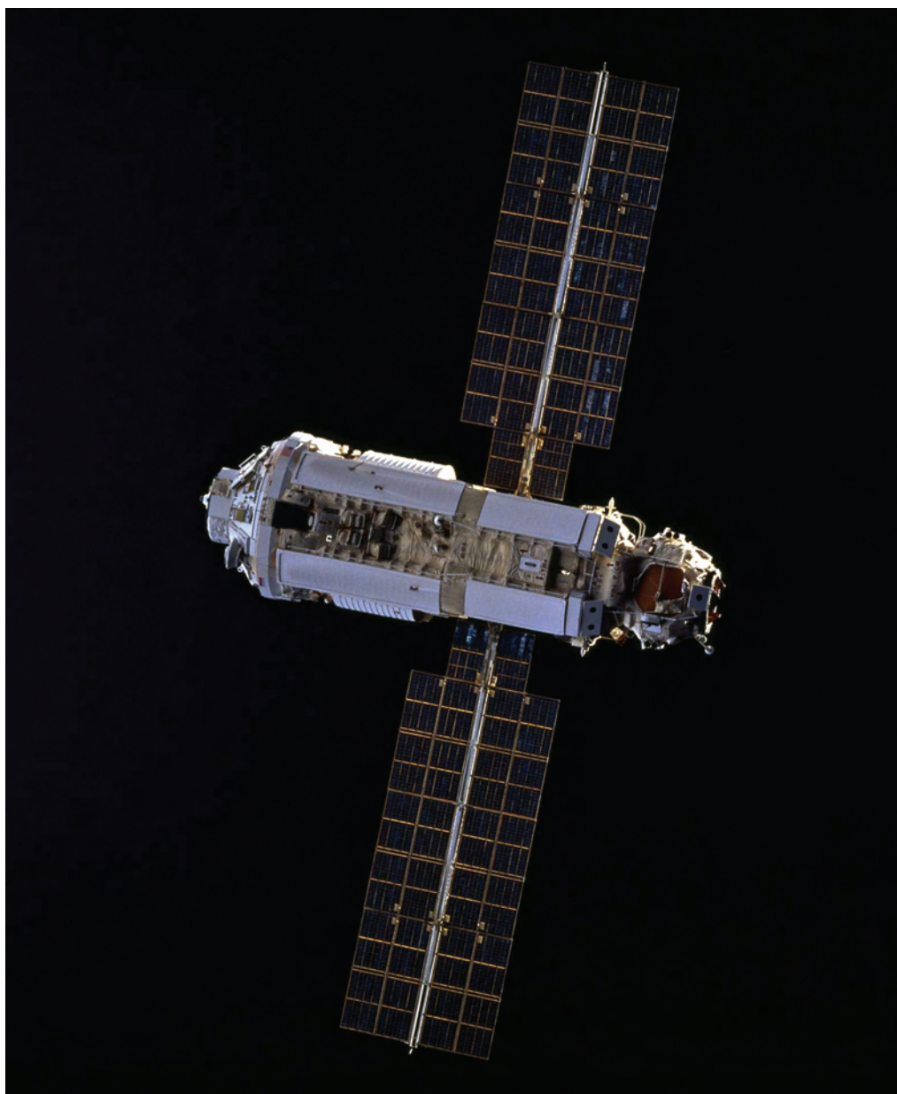
FIGURE 4.7 International Space Station functional cargo block—first element. ISS Zarya module as seen from STS-88. SOURCE: Courtesy of NASA.
