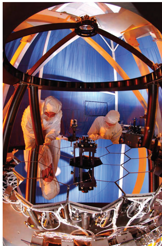
FIGURE 1.15 The JWST mirror rack. SOURCE: Courtesy of Ball Aerospace Corporation.
